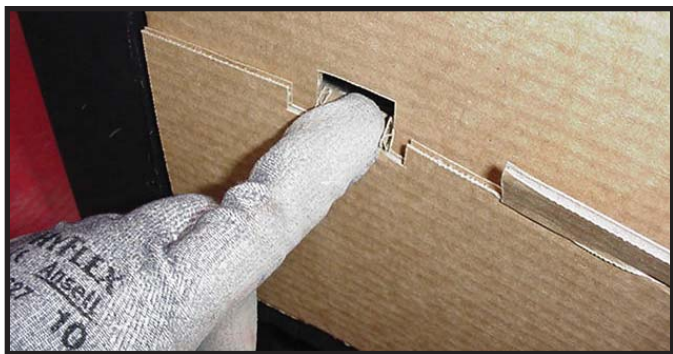
Figure 13.9 Securing Tabs Inside Front of Splatter Guard
